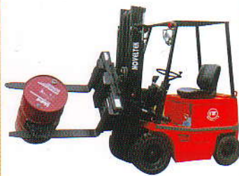
ABF-15/20/25 + ROTATING FORK CLAMP (AC)
